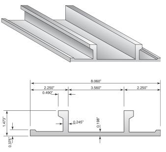
**Cross Section of Standard Vertical Rail**
