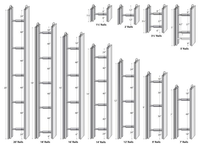
HYDRAULIC VERTICAL SHORING (Dimensions are taken from the cylinder's center lines)
