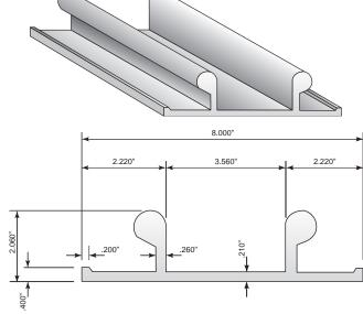
Cross Section of Heavy-Duty Vertical Rail
